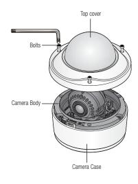
Loosen 3 screws on the camera body counter clockwise, and push down the left/right LOCKER lever (in the arrow direction) to release the lock. Then, remove the camera from the case.
